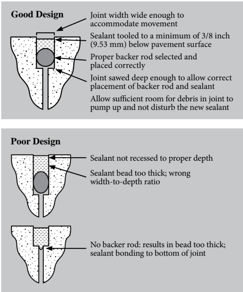
\*Recess is measured from the highest point of the installed backer material to the lowest point of the pavement surface at the joint wall.
