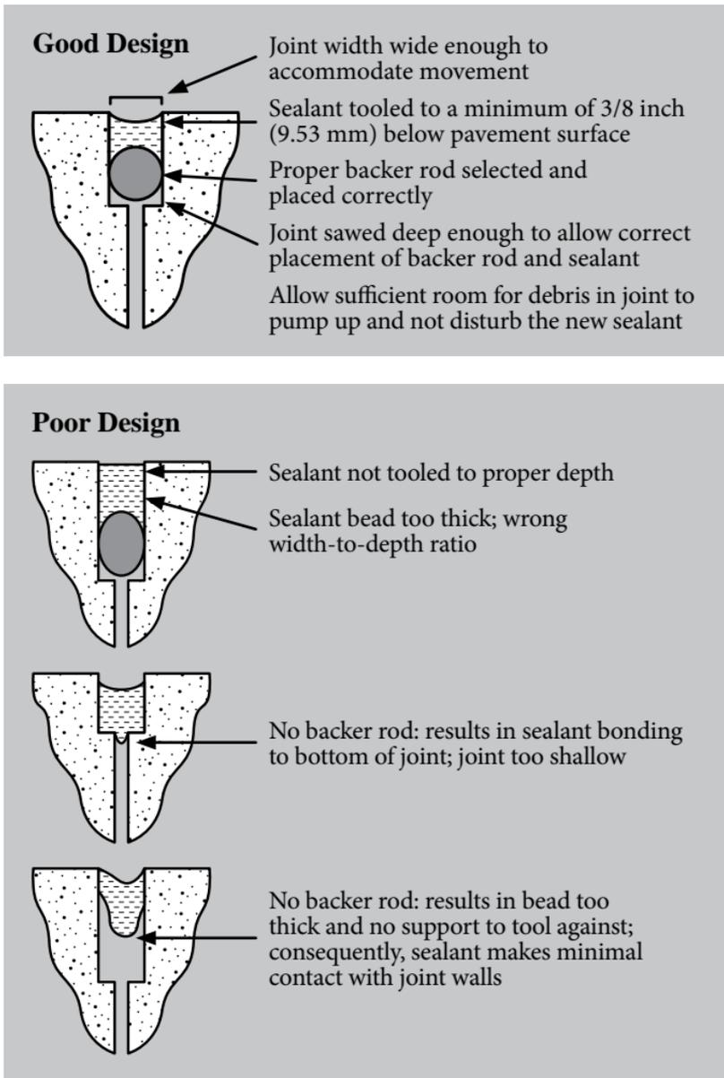
Figure 3 – Joint Design Considerations: *Dow Corning 890-SL* Silicone Joint Sealant
