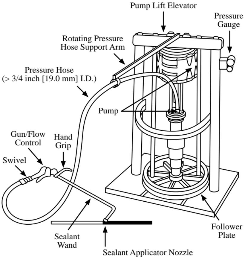
Air-powered equipment is available with varying output capacities. The ratio of the extrusion pump and accessory components of the system, especially hose diameter, will determine output volume. Specific ratios vary among manufacturers, but a ratio of 35:1 is the minimum capable of delivering a sufficient volume of sealant for efficient operation. Selection of the pump and accessory equipment should be based on desired production rates.
